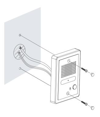
5. Place the system on the wall and mount with screws supplied.
